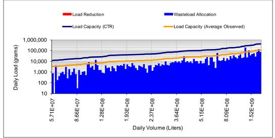
Note: The blue loading capacity line was based on the total recoverable lead concentration calculated from the dissolved CTR water quality criteria using a site-specific translator. The orange loading capacity line was calculated using the average observed total lead concentration, which represents existing conditions, and was used for TMDL calculations and allocations.
